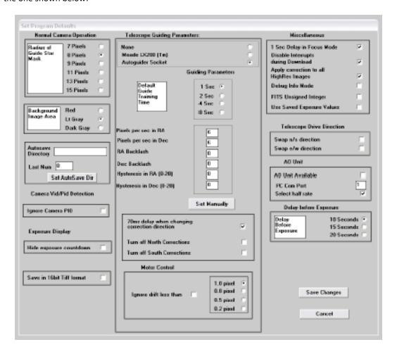
The settings shown above are generally satisfactory as a starting point, although some will probably need refinement for best results. In the example shown, the 'autoguider socket' on the Lodestar is providing the control signals to the mount, but you might alternatively use the 'LX200' mode via the
