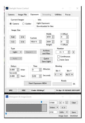
After the exposure and download have completed (about 4 seconds) an image of some kind will appear on the computer monitor. It will probably be poorly focused and incorrectly exposed, but any sort of image is good. In the case of the pinhole, all that you can experiment with is the exposure time, but a camera lens can be adjusted for good focus and so you might want to try this to judge the high image quality that it is possible to achieve.
