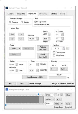
After the exposure and download have completed (about 4 seconds) an image of some kind will appear on the computer monitor. It will probably be poorly focused and incorrectly exposed, but any sort of image is good. In the case of the pinhole, all that you can experiment with is the exposure time, but a camera lens can be adjusted for good focus and so you might want to try this to judge the high image quality that it is possible to achieve.
