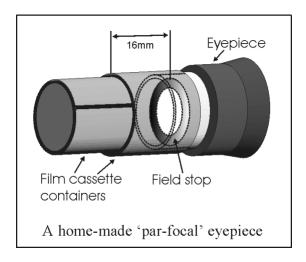
When the par-focal eyepiece is fitted into the telescope drawtube, you can adjust the focus until the view is sharply defined and the object of interest is close to the field centre. On removing the eyepiece and fitting the CCD camera, the CCD will be very close to the focal plane of the telescope and should record the stars etc. well enough for the focus to be trimmed to its optimum setting
