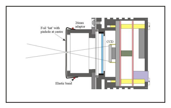
If you use a normal lens, then stop it down to the smallest aperture number possible, (usually F22), as this will minimise focus problems and keep the light level reasonable for daytime testing. The pin hole needs no such adjustments and will work immediately, although somewhat fuzzily!
