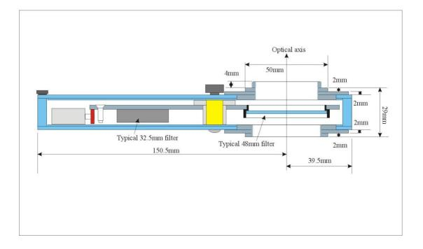
Here is a simplified cross-sectional view of the filter wheel
