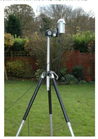
The minimum setup requires only a USB cable to the monitoring computer. This should be as short as is practical, but it will probably be necessary to have a fairly long lead if the Oculus PRO is mounted high on a mast or roof. As the camera power is taken from the 12V supply, any long leads should be as heavy as possible to reduce the internal resistance. The USB2.0 cable should be kept to a minimum and if an extension is required, a high quality USB active extension cable should be used.
