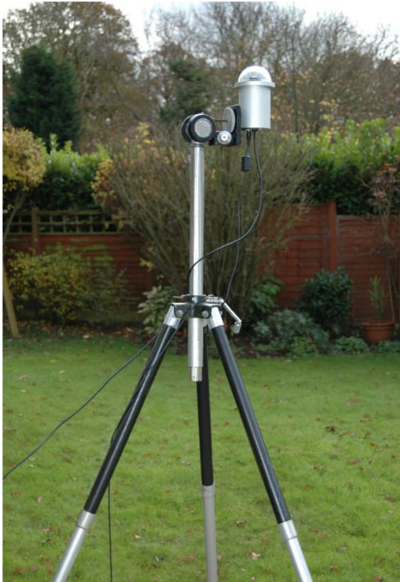
A simple setup with the Oculus mounted on an old tripod
