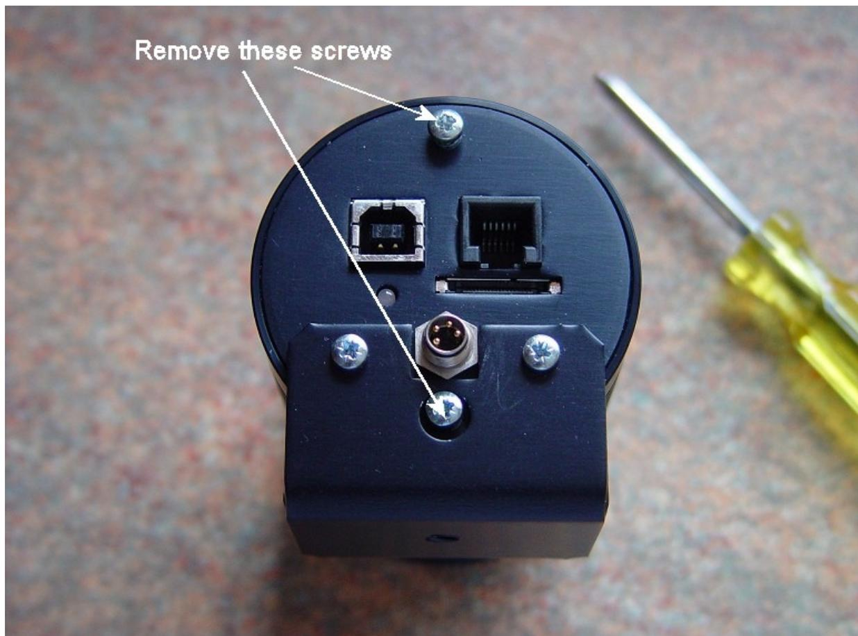
Lift off the back plate (wiggle it off the USB plug) and expose the power lead:
