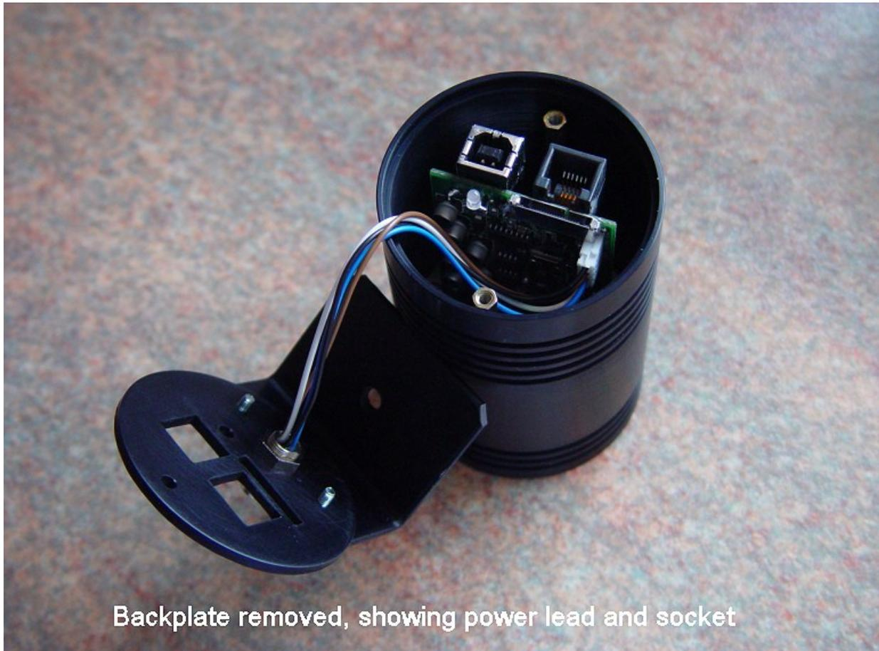
Backplate removed, showing power lead and socket
